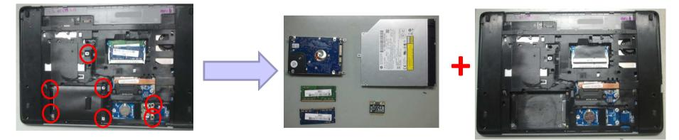
Loose HDD & ODD module screws and take off HDD & ODD module from system. Loose WLAN/WWAN screws and take off WLAN/WWAN,DIMM module from system.
